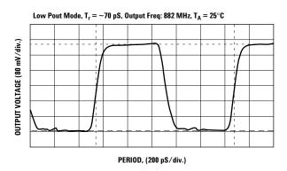
Figure 6. Typical Output Voltage Waveform.
