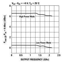
Figure 7. Typical Output Power vs. Output Frequency,  $f_{\rm out}$  (GHz).
