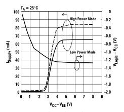
Figure 5. Typical Supply Current &  $V_{Logic}$  vs. Supply Voltage.
