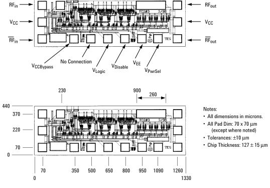
Figure 2. Pad Locations and Chip Dimensions.
