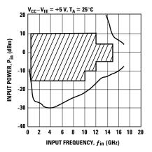
Figure 4. Typical Input Sensitivity Window.
